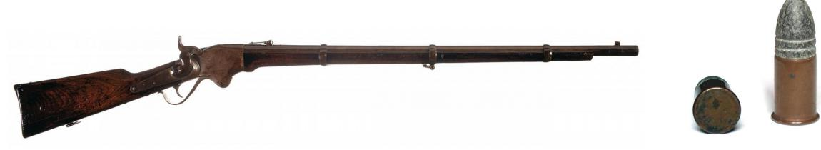
Christopher Spencer invented a lever action repeating rifle in about 1860. The Spencer Rifle fired a .52 caliber metallic cartridge from a magazine tube holding 7 rounds. The Rifle was 47" long with a 30" barrel and was also produced in a 39.25" Carbine version. The rifle weighed in at 10 pounds.
